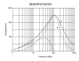
The chip ferrite beads BLM series is designed to function nearly as a resistor at noise frequencies, which greatly reduces the possibility of resonance and leaves signal wave forms undistorted.
