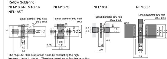
frequency noise to ground. Therefore, to get enough noise reduction, feed through holes which are connected to ground-plane should be arranged according to the figure to reinforce the ground pattern.
