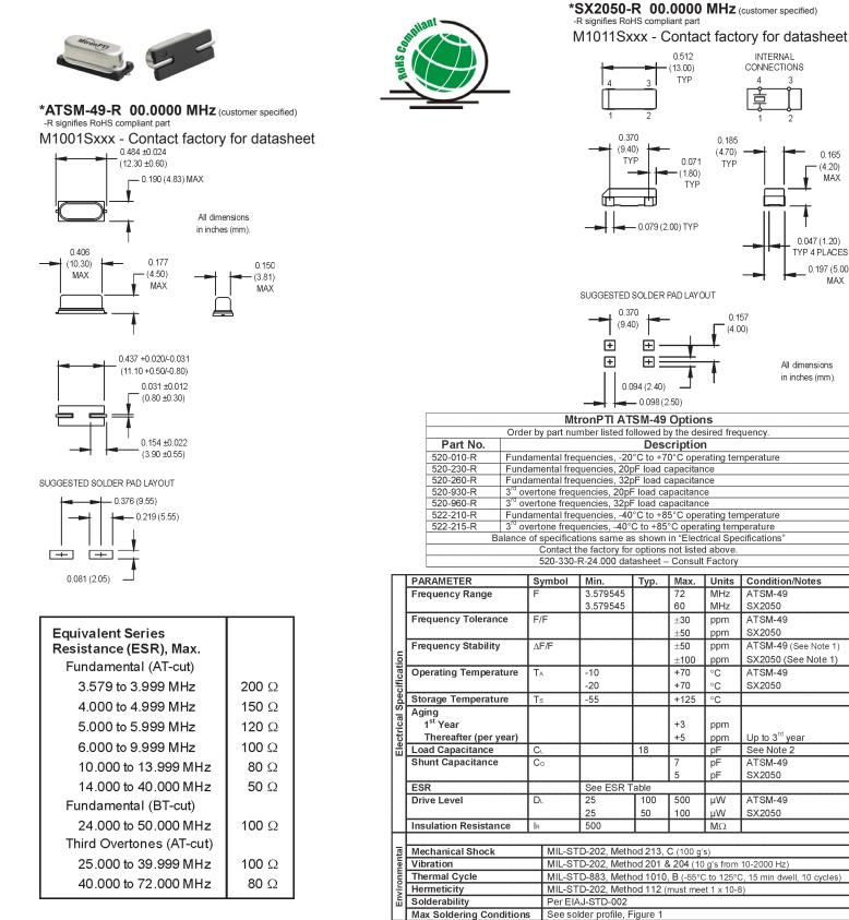
Note 1: BT Cut fundamentals from 24,000 to 40,000 MHz have a stability of  $\pm 100$  ppm Note 2: Series resonant designated by "SR" prefix (ie., SRATSM-49 or SRSX2050
