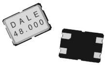
The XT57C is a miniature SMD crystal with 7.0 x 5.0 ceramic package and a height of 1.1 mm maximum. 9.8304 MHz to 100 MHz frequency makes it widely applied in notebook computer, PCMCIA, and communication equipment.
