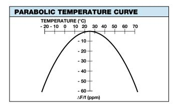
To determine frequency stability, use parabolic curvature (k).
