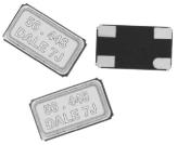
This part is an ultra miniature package with size of  $6.0~\text{mm} \times 3.5~\text{mm} \times 1.0~\text{mm}$ . With its ceramic base and metal cover it provides the durability and reliability necessary for strenuous process like infrared and vapor phase reflow.
