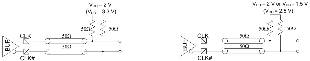
Figure 9. LVPECL Termination
