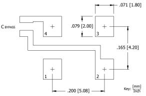
$C_{BYPASS}$  should be  $\geq 0.01$  uF.
