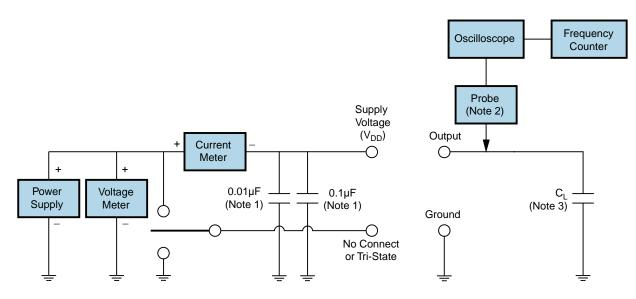
Note 1: An external  $0.1\mu$ F low frequency tantalum bypass capacitor in parallel with a  $0.01\mu$ F high frequency ceramic bypass capacitor close to the package ground and V<sub>DD</sub> pin is required.
