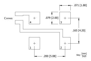
$C_{\text{RYPASS}}$  should be  $\geq$  0.01 uF.
