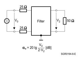
Symmetrical measurement circuit with  $Z_{\text{L}}$  = 50  $\Omega$
