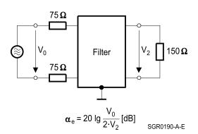
Symmetrical measurement circuit with  $Z_{\text{L}}$  = 150  $\Omega$
