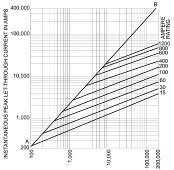
RMS SYMMETRICAL CURRENTS IN AMPERES A-B = ASYMMETRICAL AVAILABLE PEAK  $(2.3 \times \text{SYMM RMS AMPS})$
