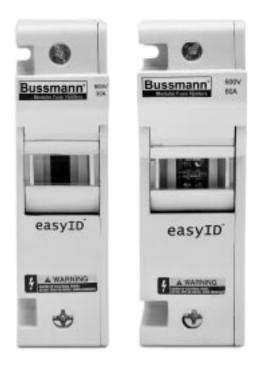
Catalog Symbol: CH30J\_(I) CH60J\_ (I) Ampere Rating: 1 to 60A Voltage Rating: 600Vac (or less) Interrupting Rating: 200,000A RMS Sym. Agency Approvals: Listed UL 512, Guide IZLT, File E14853 CSA Certified per C22.2 Nos. 39 Class 6225-01, File LR47235
