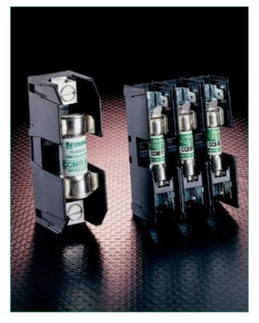
Space saving 600 volt, 30 amp molded case fuse blocks with side barriers for isolation. Class CC blocks and Midget blocks are identical except Class CC blocks incorporate a rejection feature to assure proper fusing.
