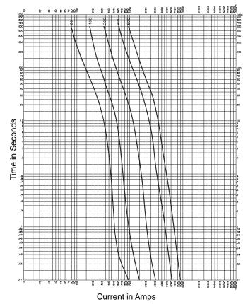
**Note:** 60 Amp fuse curve is ferrule style and included to show only relative performance. For actual 60 amp time-current curve performance, see Data Sheet 1003.
