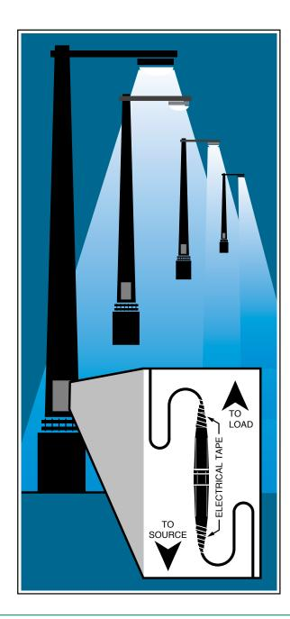
Littelfuse 600 volt in-line watertight fuse holders are the ideal answer for all high humidity and corrosive environments where fuses are required. Available in both breakaway and non-breakaway, single and double pole versions, these fuseholders allow maximum flexibility for any application.
