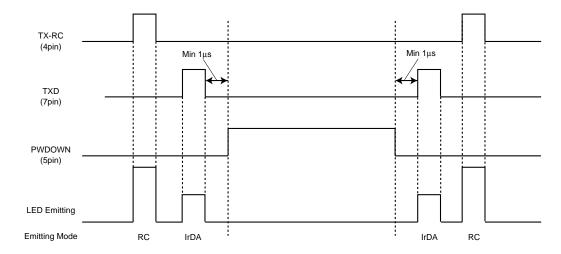
$* If TX-RC \ or \ TXD \ input \ pulse \ width \ is \ wider \ than \ 48 \mu s, \ output \ LED \ emitting \ pulse \ will \ be \ turn \ off \ approximately \ 48 \mu s.$
