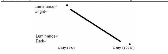
2) ADJ signal =0~3.3V, operation frequency:20KHZ±5KHz
