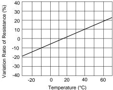
The variation ratio of the temperature coefficient will be comparatively larger with weak measuring light. The resistance value will increase as the ambient temperature goes up.
