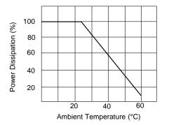
Tolerable power dissipation is the permissible amount of power the cell may dissipate when it is employed in a given circuit. This value is dependent on the characteristics of the photoconductive cell itself and is external covering in relation to ambient temperature and generated temperature all cells are measured at 25°C.
