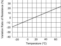
The variation ratio of the temperature coefficient will be comparatively larger with week measuring light. The resistance value will increase as the ambient temperature goes up.
