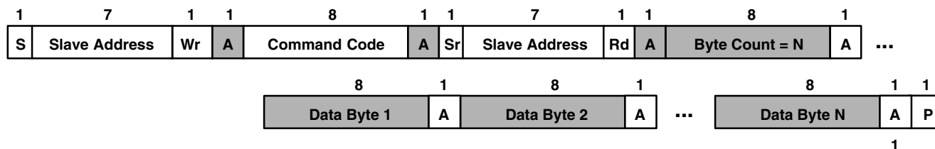
Figure 19. SMBus Block Read or I²C Read (Combined Format) Protocols
