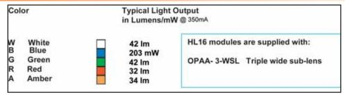
Results are LED manufacturer's test data @ 25°C JTC'. Light output at 55°C PCB temperature will be approximately 15-20% lower. Elevated temperatures will result in further degradation of light output. For maximum performance use appropriate heat sinking.
