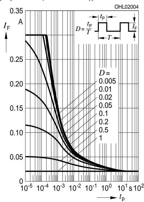
**Zulässige Impulsbelastbarkeit  $I_F = f(t_p)$** **Permissible Pulse Handling Capability**Duty cycle  $D$  = parameter,  $T_A = 85^\circ\text{C}$
