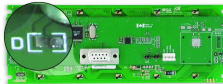
Figure 12: Power Through DB-9 Jumper
