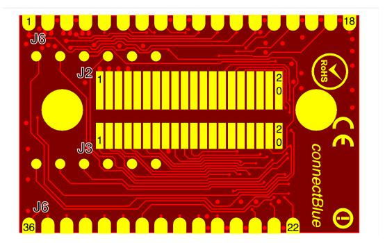
Solder lands connector (J6) has a new layout compared to cB-OWSPA311g.
