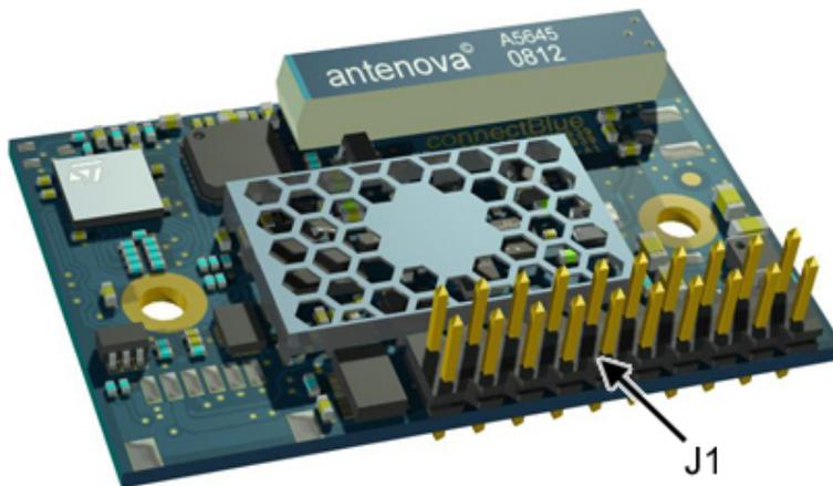
Figure 4: The 2x20 2mm pin header connector (J1) mounted on the module (cB-OBS433i-02).
