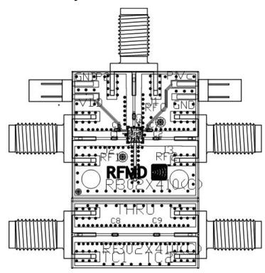
Broadband Application Circuit (500MHz to 4000MHz) - all capacitors are 100pF. Operation outside this band requires re-optimization of the capacitors.
