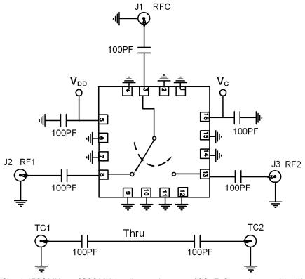
Broadband Application Circuit (500 MHz to 4000 MHz) - all capacitors are 100 pF. Operation outside this band requires re-optimization of the capacitors.
