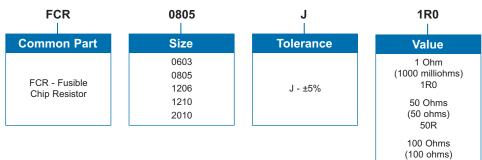
Dimensions are in millimetres unless otherwise specified. 100R
