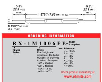
These Hi-Meg resistors are designed for use in electrometer circuits where a high order of performance is required. These resistors achieve a high degree of accuracy and stability, and operate at this high performance level for an extended period of time. By being vacuum sealed in a glass envelope, these Hi-Megs are suitable for ultra-high vacuum applications.
