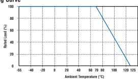
For temperatures in excess of 70°C the load shall be derated in accordance with this curve.
