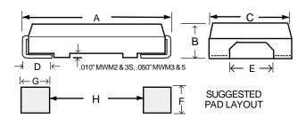
Exceptional perfomance and reliability is achieved via highest grade materials and processing. An all-welded wirewound construction is standard, featuring premium-grade wire for superior stability and surge capability. Opt. L low profile models feature a non-inductive metal plate element. The power film version (Opt.M) achieves values as high
