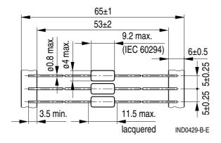
Minimum lead spacing 12.5 mm
