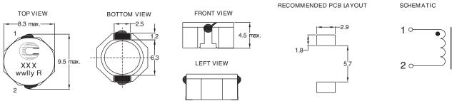
Dimensions are in millimeters.
