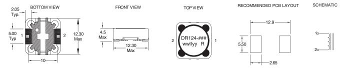
Dimensions are in millimeters.
