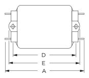
.250 [6.3] with .07 [1.8] Dia. hole .250 [6.3] with .07 x .16 [1.8 x 3.8] slot
