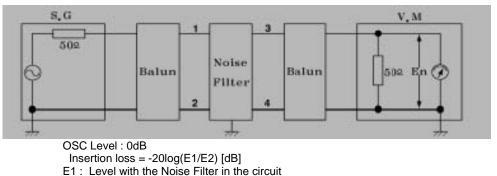
E2: Level without the Noise Filter in the circuit
