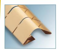
high deflection no-snag, fold-under WITH ADHESIVE MOUNT. For applications requiring low compression force. Designed with a minimum residual stress and highly leveraged spring action. The free end features a fold-under lip which facilitates a low coefficient of friction on most surfaces. Allows a minimum of compressive force to move through the deflection range, resulting in the highest levels of shielding effectiveness with a minimum force.
