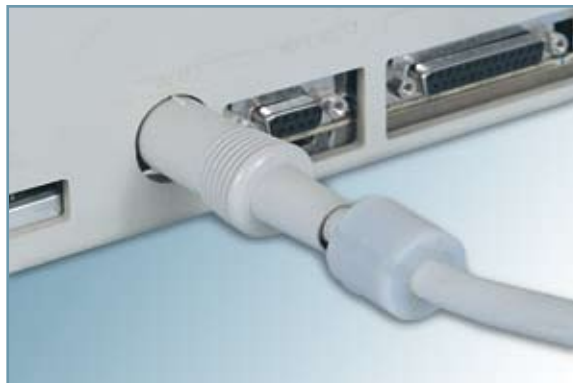
I/O cable with RFI suppressor.
