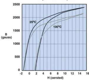
Measured on a 19/10/6mm toroid at 10kHz.
