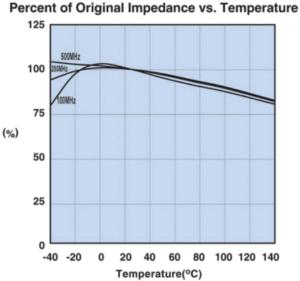
Measured on a 2661000301 using the HP4291A.
