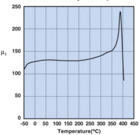
Measured on a 19/10/6mm toroid at 100kHz.
