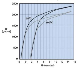
Measured on a 19/10/6mm toroid at 10kHz.
