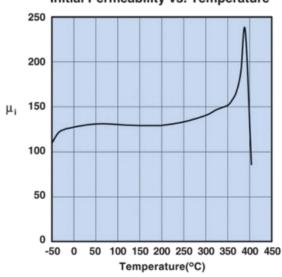
Measured on a 19/10/6mm toroid at 100kHz.
