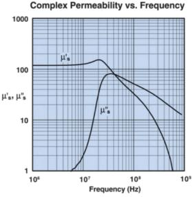
Measured on a 19/10/6mm toroid using the HP 4284A and the HP 4291A.
