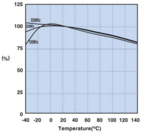
Measured on a 2661000301 using the HP4291A.
