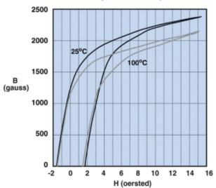
Measured on a 19/10/6mm toroid at 10kHz.
