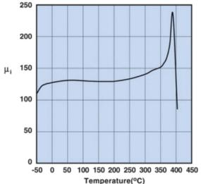
Measured on a 19/10/6mm toroid at 100kHz.
