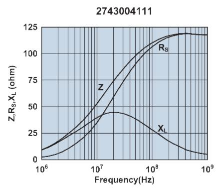
Impedance, reactance, and resistance vs. frequency.
