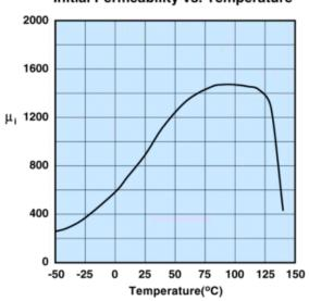
Measured on a 17/10/6mm toroid at 100kHz.
