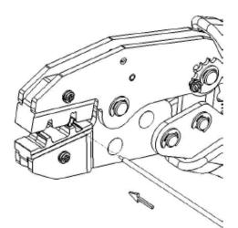
Then, insert the cable into the open barrel. After that, squeeze the handle at the till ratchet released.
