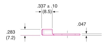
Max Electric Current: 8 AWG / 62 Amp
