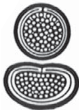
Strands enter as a homogeneous group and compact tightly under compression due to fully brazed seam
