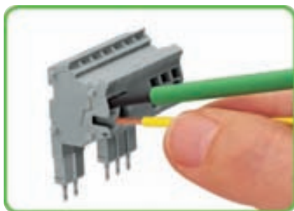
Wire connection: Screwdriver actuation for connection of all conductor types, i.e. stripped stranded conductors, or push-in connection of solid or ferruled stranded conductors.
