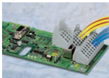
Removing the terminal blocks to place the board
