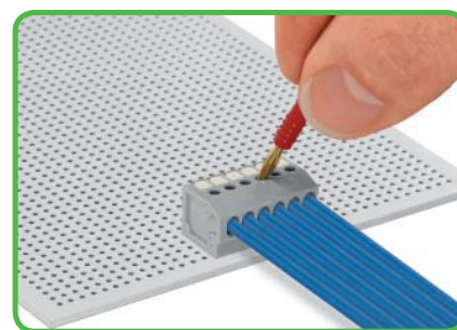
Testing with test plug Ø 2 mm/0.079 in. Insert the test plug slightly inclined into the test slot
