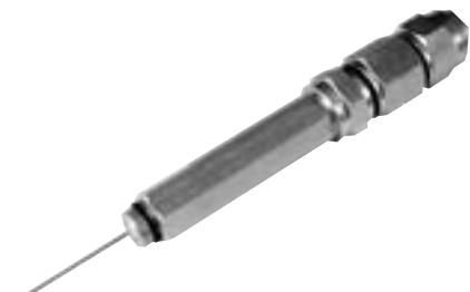
5/8" – 24 3 piece extended entry connectors with auto seize technology for enhanced cable seizure. 2" pin and center conductor cutting guide are standard. Common hex size per connector with tapered back nut for consistent heat shrink application. Re-enterable and reusable. Three piece design allows visual inspection of connector and cable during installation. Available in 3", 6" and 9" lengths.
