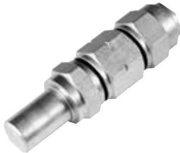
3 piece cable terminator. Blocks 60 Hz AC power and terminates RF signal. Auto seize technology for enhanced cable seizure. Center conductor cutting guide is standard. Common hex size per connector with tapered back nut for consistent heat shrink application. Three piece design allows visual inspection of connector and cable during installation. Re-enterable and reusable.
