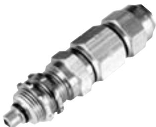
3 piece cable to "F" female adaptor capable of being secured in place for permanent mounting. Auto seize technology for enhanced cable seizure. Center conductor cutting guide is standard. Common hex size per connector with tapered back nut for consistent heat shrink application. Three piece design allows visual inspection of connector and cable during installation. Re-enterable and reusable.
