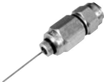
5/8"- 24 2 piece pin type entry connector with auto seize technology for enhanced cable seizure. 2" pin and center conductor cutting guide are standard. Common hex size per connector with tapered back nut for consistent heat shrink application. Re-enterable and reusable.
