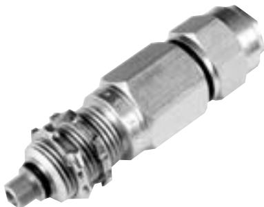
2 piece cable to "F" female adaptor capable of being secured in place for permanent mounting. Auto seize technology for enhanced cable seizure. Center conductor cutting guide is standard. Common hex size per connector with tapered back nut for consistent heat shrink application. Re-enterable and reusable.
