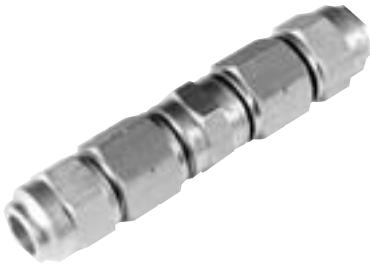
Connectors to join two identical cables together. Auto seize technology incorporated in both connector ends assures best possible connection. Three piece design allows visual inspection of connector and cable during installation. Common hex size per connector with tapered back nut for consistent heat shrink application. Connectors are re-enterable and reusable with integrated center conductor cutting guide.
