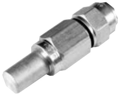
2 piece cable terminator. Blocks 60 Hz AC power and terminates RF signal. Auto seize technology for enhanced cable seizure. Center conductor cutting guide is standard. Common hex size per connector with tapered back nut for consistent heat shrink application. Re-enterable and reusable.
