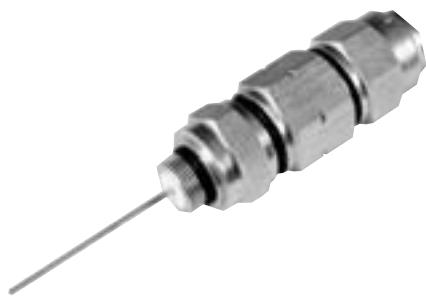
5/8"- 24 3 piece pin type entry connector with auto seize technology for enhanced cable seizure. 2" pin and center conductor cutting guide are standard. Common hex size per connector with tapered back nut for consistent heat shrink application. Re-enterable and reusable; three piece design allows visual inspection of connector and cable during attachment.
