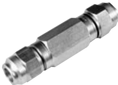
Connectors to join two identical cables together. Auto seize technology incorporated in both connector ends assures best possible connection. Splice connectors are re-enterable and reusable with integrated center conductor cutting guide. Common hex size per connector with tapered back nut for consistent heat shrink application.
