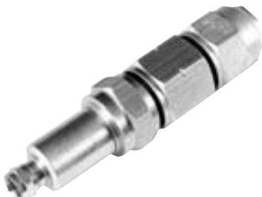
3 piece cable to "F" male adaptor. Auto seize technology for enhanced cable seizure. Center conductor cutting guide is standard. Common hex size per connector with tapered back nut for consistent heat shrink application. Three piece design allows visual inspection of connector and cable during installation. Re-enterable and reusable.
