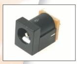
DC-9 PCB mounting pin ring type with switch. Rated 12V / 5A. DC9 with 2.1mm dia. pin. DC9A with 2.5mm dia. pin.
