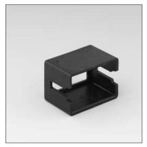
When pins are inserted into the panelmount receptacle half (SMS--R1) of the QIKMATE connector, an optional pin protection shroud can be installed. The shroud is mounted at the same time as the receptacle by holding the shroud against the mating side of the panel with both cutouts lined up. The receptacle is then inserted in place, trapping the shroud between the receptacle and panel. The use
