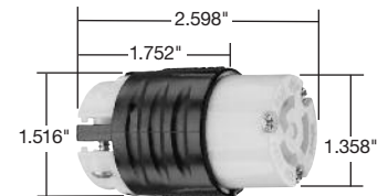
Dimensions for 15 Amp Connector
